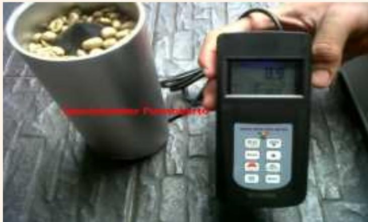
Gambar 5. Moisture tester seri SM1701M.
